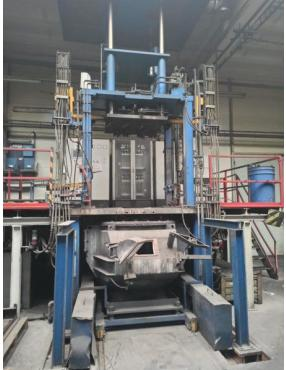
A large industrial casting machine, specifically a low-pressure casting machine (Kurtz AL 16-12 SR ND1349), is shown in a factory setting. The machine is a complex assembly of blue-painted metal frames, hydraulic systems, and control panels. It appears to be in an operational state, with various components like molds and conveyor belts visible. | <b>1,00 €</b>   |
